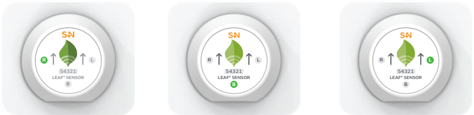
Figure 10: LEAF Patient Sensor LED scrolling pattern
