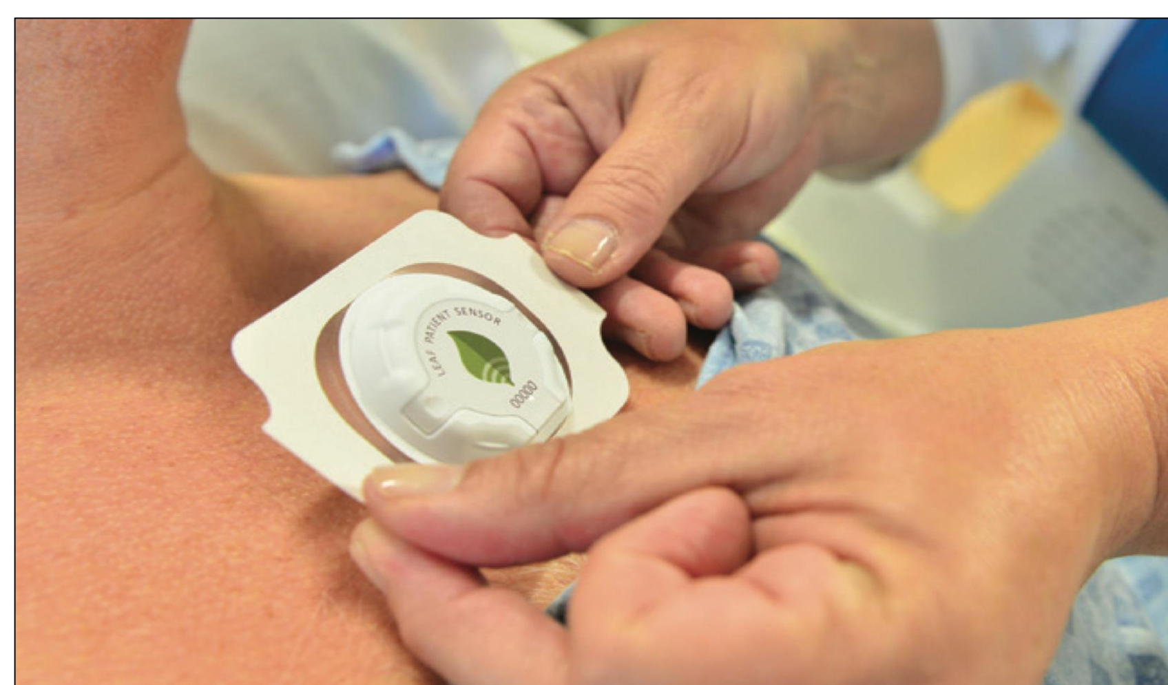
A sensor is applied to a patient's upper torso. The sensor continuously monitors the patient's movement and position. Sensor data is wirelessly communicated through a network of relay antennas and viewable on computers, TVs, and mobile devices.
